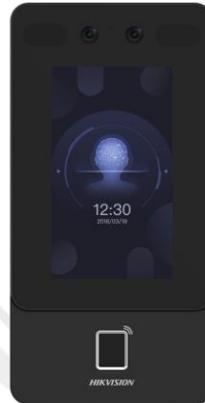
Face recognition terminal adopts deep learning algorithm, which helps to recognize the face faster with higher accuracy. It also supports multiple authentication modes: face/card/fingerprint authentication, etc. It can be applied in multiple scenarios, such as buildings, enterprises, financial industries, and other important areas.
