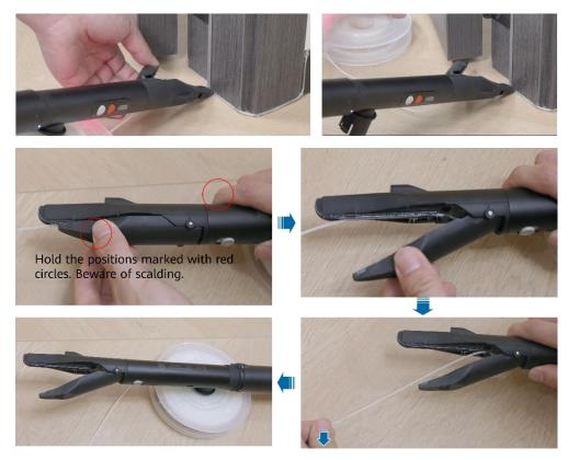
Step 2 Route the transparent optical cable through the door gap.
