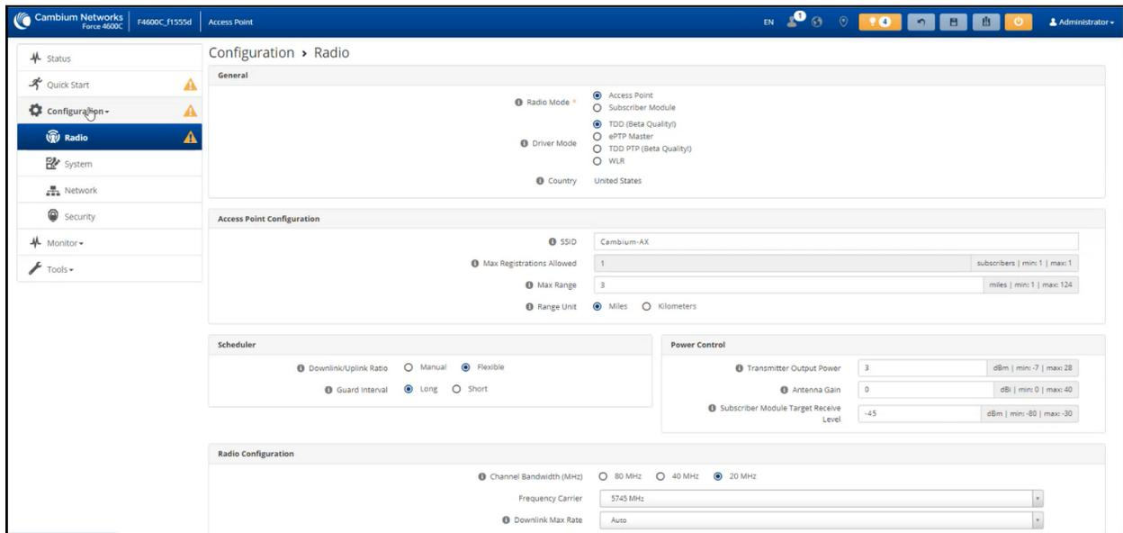
Figure 10: Configuration > Radio page (AP mode)
