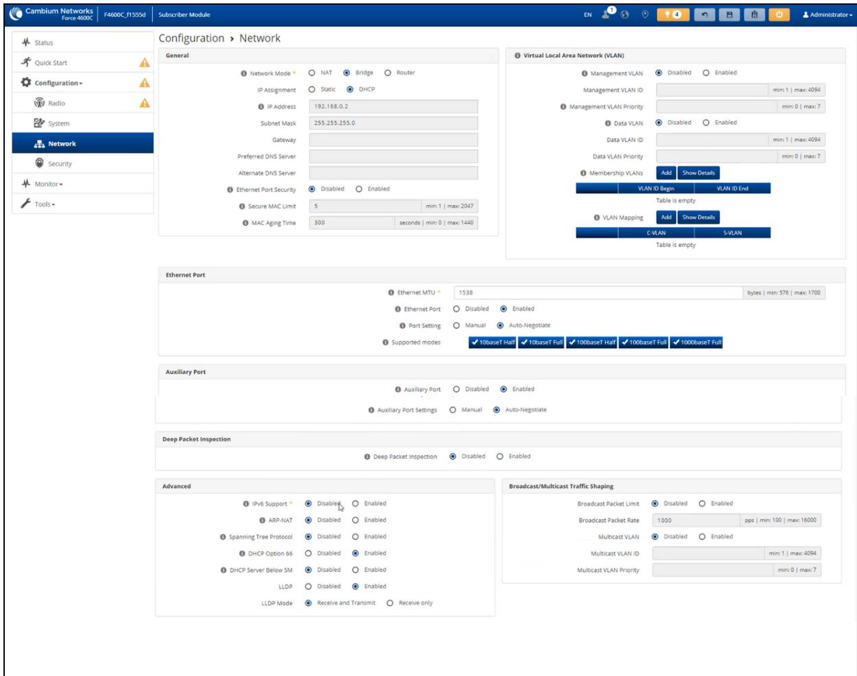
Figure 16: Configuration > Network page (SM mode, Bridge Network mode)
