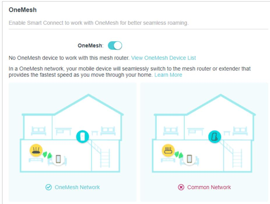
4. Connect a OneMesh extender to this router by following the setup instructions in the extender's manual. The extender will be listed on the router's [OneMesh](#) page.
