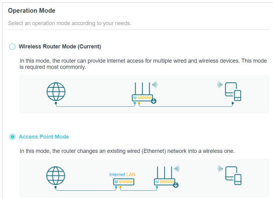
3. After rebooting, connect the router's WAN port to your existing wired router's LAN port via an Ethernet cable.
