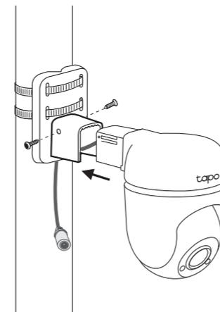
\*Pole-mounting loops are not included. Prepare the required accessories for pole mounting in advance.
