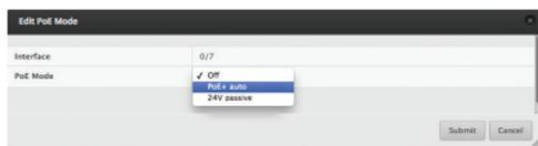
**Note:** If the *PoE* screen states that PoE is not supported, then there is insufficient power. You will need to increase the power input to the EdgePoint.
