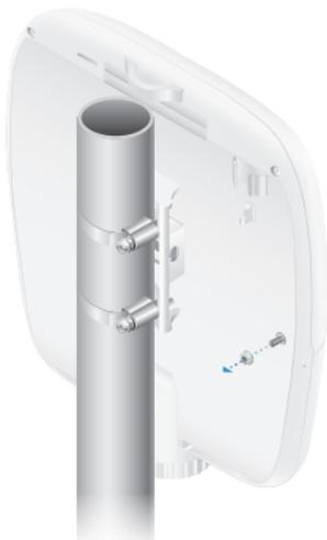
2. Attach a ground wire (min. 10 AWG or 5 mm<sup>2</sup>) to the lug and replace the nut to secure the wire.
