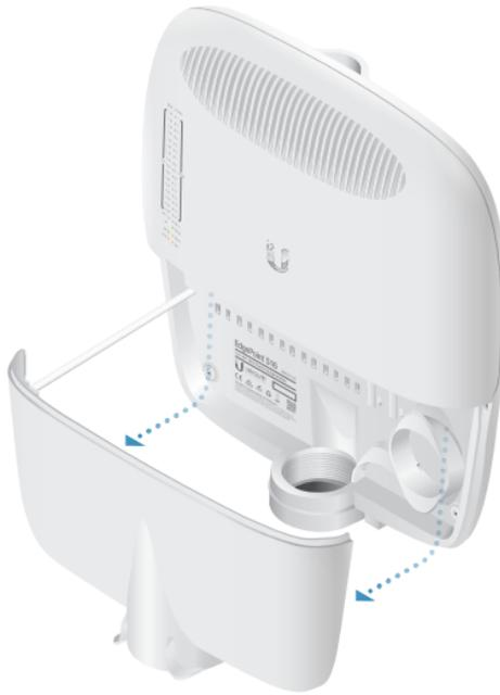
2. Feed the Ethernet cables through the *Cable Sleeve* and connect them to ports in this range: 1-16.
