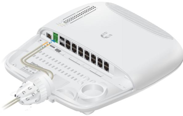
2. Replace the port cover and use an S2 hex wrench to tighten the Screw and secure the port cover.
