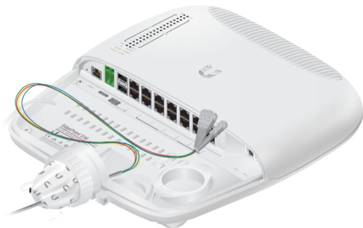
3. Separate the fiber optic strands and spool them around the strain relief reels in the direction of the arrows. Then connect a fiber optic strand to the fiber module.
