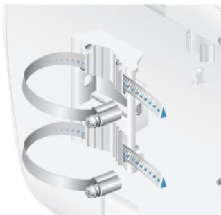
2. Wrap the *Metal Straps* around the pole. Use a 7 mm socket wrench to turn the screws clockwise and securely fasten the straps to the pole.
