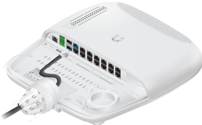
3. You can create a strain relief for any Ethernet cable by feeding a cable tie (not included) through the tie slot under the cable. Then wrap the cable tie around the cable and tighten.
