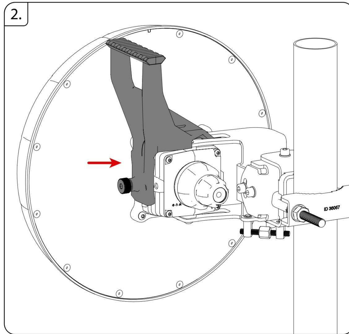
2. Slide nRAYAIM on the nRAY body as it is shown in the picture until it stops in position.
