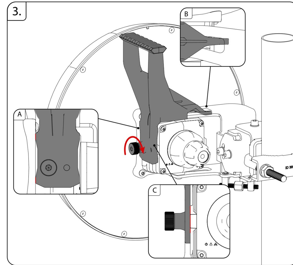
3. Secure the mount with the included screw. Make sure that the nRAYAIM is positioned correctly: A) two edges lean against the product body; B) The nRAYAIM tail is attached under the pole mount; C) The nRAYAIM surface is in level with the shown surface.
