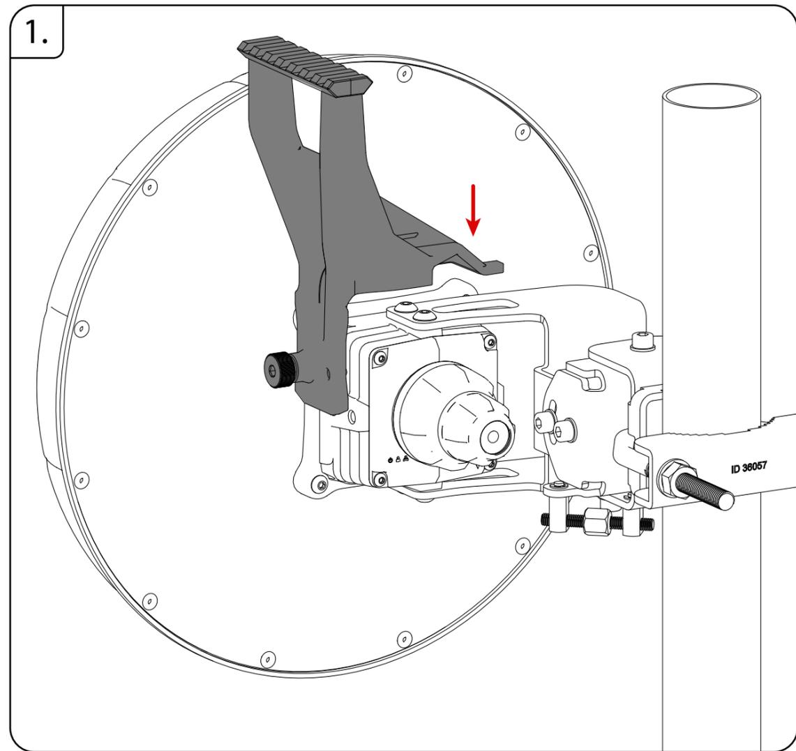
1. Attach the nRAYAIM onto nRAY body as it is shown in the picture.
