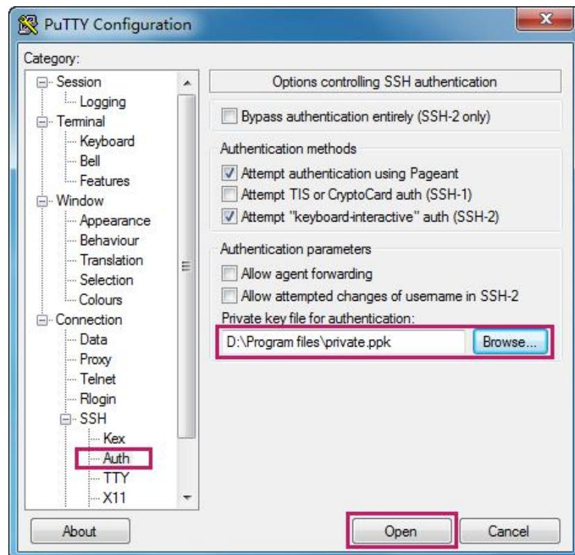
After successful authentication, enter the user name. If you log on to the device without entering password, it indicates that the key has been successfully downloaded.
